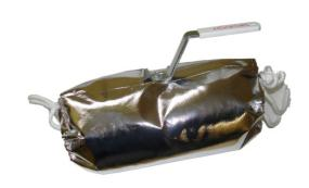
CeeVee Ltd provides flexible, removable and reusable Insulation jackets designed to fit the Hogfors Fig 34500TR range of ball valves, which allow for easy accessibility for inspection or replacement. Each jacket has two layers of heat & flame resistant cloth enclosing a layer of insulating material, complete with fire retardant Velcro ™ & string fasteners for simple installation and removability.
