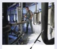
Foam Lance Ensures a thick and consistent application on all surfaces which increases the efficiency of the chemical
