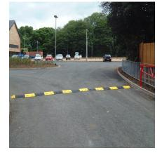
The AUTOPA Speed Ramps are fully modular and created from a variety of sections, each are sold separately allowing for any length of speed ramp. All shoulders and inners are available in black or yellow and the chart below will determine the correct number of each required for your site.
