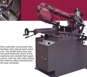
bandsaw with manual quick action vice. The S200R heavy duty saw has electrohydraulic return of the sawframe and variable feed speed control, with two way mitre cutting this machine offers everything for the busy workshop.
