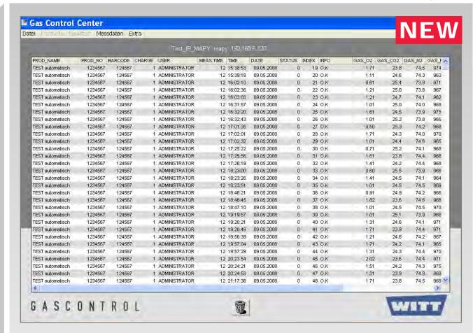
Windows-Software for the documentation of analysis-results of OXYBABY®6.0 /-Med, MAPY, LEAK-MASTER®, MAPMAX and other WITT- equipment with integated or separate analysis.
