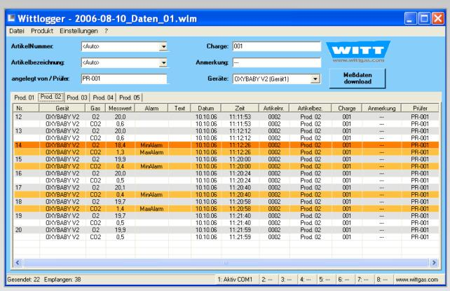
Windows-Software for the documentation of analysis-results of OXYBABY®6.0, MFA, PA and other WITT- equipment with control system (AWS).
