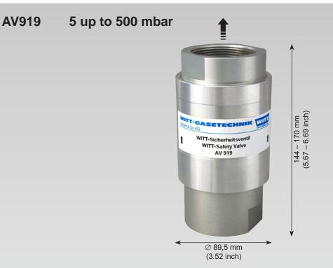
Spring loaded, direct acting safety relief valve for venting excess pressure from receivers, pipelines and other equipment.
