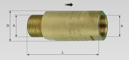
SRV - Safety valve consisting of a non-return valve and a thermal device to shut off oxygen in case of backfire.
