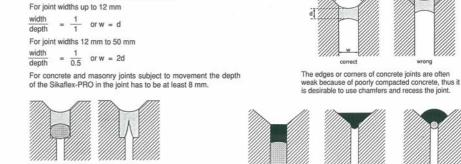
The "bottom" of the joint must not restrict the deformation of the sealant since this could result in failure during the opening of the joint. The depth of the joint should be adjusted by incretines withhole licits the deformation to the sealant since the inserting a suitable joint backing material.
