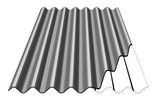
The cut-away illustration above shows the location of the polypropylene reinforcement strip inserted in a precisely engineered position in each corrugation of the Profile 6 sheet.
