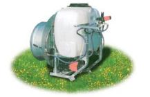
HOT GALVANIZED TUBULAR FRAME, THREE POINTS LINKAGE (TYPE 0 OR SMALLER), 200 LITRE POLYETHYLENE TANK WITH HANDWASH TANK external suction filter, anti-pollution ejector, remote pressure regulator. Hot galvanized fan diam 550 mm with adjustable blades, one speed gear box with declutch and neutral position, stainless steel nozzles holder staffs, brass nozzles with anti-drip with ceramic nozzles. MACHINE SIZE: 85x120x130 cm
