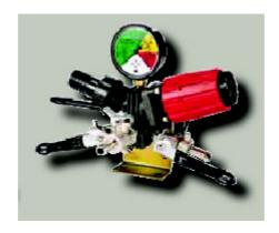
The control unit allows pump pressure to be adjusted, the pressure to be controlled by means of a special pressure gauge as well a flow on and off controls by turning the lever. For information see the booklet use and maintenance of control units.
