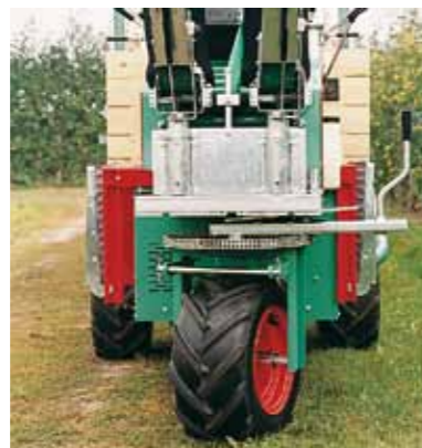
The steering wheel of the Pluk-O-Trak Junior can be easily adjusted to the left, right or centre. This means that it is always within easy reach, even when pickers are working on side rows.
