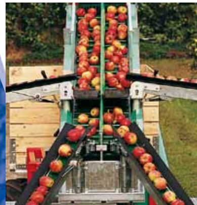
The picking belts, the main conveyor belt and the bin filler operate independently of the driving speed of the machine.
