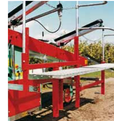
Pluk-O-Trak Senior: two picking platforms on each side and hydraulic steering
