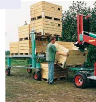
Pluk-O-Trak Senior: two picking platforms on each side and hydraulic steering
