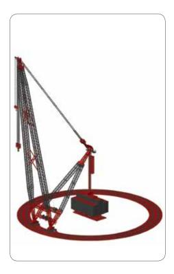
The AL.SK350 is being built to accommodate a long term project based in Brazil, it will have a maximum lifting capacity of 5,000te using the strand jack system and is also fitted with a 2,000te winch system. It has a load moment of 354,000tm (which is some 77% higher than its nearest rival), and a main mast length of 141.2m. It can also be fitted with a fixed 120m jib.
