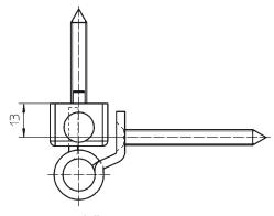
RB 5020 3D – drilling position 13.0 mm
