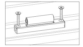
2 Mount door part with positioning cams in the sash holes and fix it by using enclosed screws (6.3 x 60 mm) (max. torque 6 Nm).
