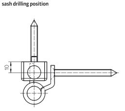
RB 5010 3D – drilling position 10.0 mm
