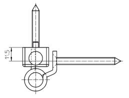
RB 5015 3D – drilling position 11.5 mm
