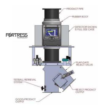
Also... a search head can be configured to operate in '*Pipeline*' mode, where the product is generally pumped through the system (shown below) and contamination is diverted away from the product flow through the '*Reject Valve*'.
