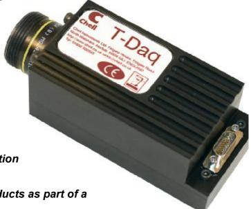
The Chell T-daq is an intelligent thermocouple temperature scanner capable of acquiring the outputs of K and E type thermocouples. It can be used in place of a PSI pressure scanner or in conjunction with the Chell CANdaq or QUADdaq products to provide a complete data acquisition system.
