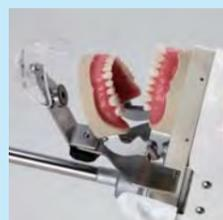
1) Loosen the adjusting screw in the back and slide down the stopper plate. Then attach the upper jaw.
