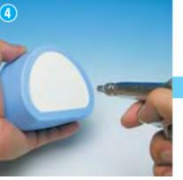
Blow air around the mold and gently remove the mold.
