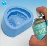
Lightly spray wax pattern cleaner or debubbler to prevent air bubbles from forming.
