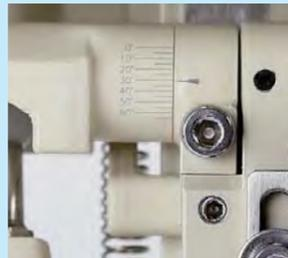
② Dial allows intricate adjustment of the jaw angle and position. The angle can be adjusted from 0°-60°.
