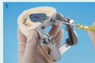
Lightly tighten the 2 screws on the upper jaw.
