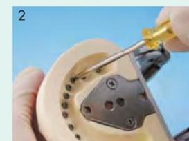
Using the supplied screwdriver, lightly screw in the fixing screw from the underside of the jaw model.
