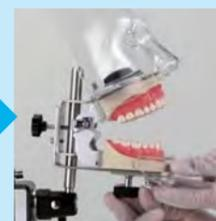
3) Pull back the chin plate and tighten the chin plate adjusting screw.
