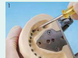
Unscrew the fixing screw on the underside of the jaw model using the supplied screwdriver.
