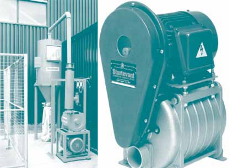
Typical vacuum cleaning system with 6X7 Turbo exhauster driven by 11Kw motor, providing the suction power.
