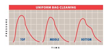
In the MCF, each filter bag is cleaned once and only once per cycle to optimise bag life and pressure drop. The use of round filter bags contributes to the exceptionally uniform cleaning achieved.
