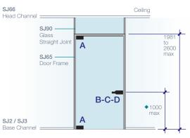
LMG19.83 - SJ65 door frame: 838 x 1981mm max height <u>or</u> LMG26.90 - SJ65 door frame: 900 x 2600mm max height
