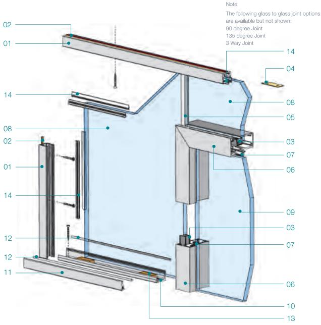
Crystal clear dry jointed system with square aluminium sections
