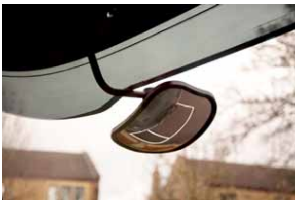
The white lines show the area of visibility required from the front view mirror on a new truck
