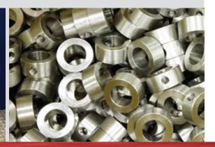
E/M Coating Services can now offer a complete vapour degreasing service carried out to the highest standards using the latest computer controlled technology. Vapour degreasing is ideal as a pretreatment to coating or welding.
