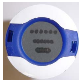
Typical Test Result – Oil present at a concentration of greater than 0.5 mg/m 3 but less than 1.0 mg/m 3
