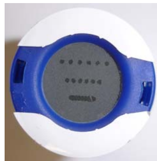
Typical Test Result – Oil present at a concentration of greater than 0.1 mg/m 3 but less than 0.5 mg/m 3
