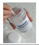
Ensure the oil tube is kept vertical throughout this process
