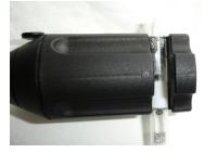
2. With one hand holding the cutter and the other holding the tube. With your thumb against the base of the cutter, apply pressure to the tube. This should break the inner tube.
