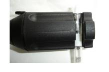
2. With one hand holding the cutter and the other holding the tube. With your thumb against the base of the cutter, apply pressure to the tube. This should break the inner tube.
