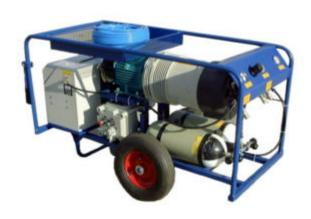
With the low running temperatures of the rotary vane compressor they can be produced to operate in hazardous atmospheres for both Zone I and Zone II applications. Sets can be modified for mobile applications with mains isolators and circuit breaker protection.
