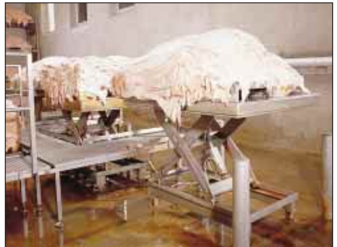
A number of 1,200Kg capacity lift tables being used in a process hall. The environment is extremely aggressive due to concentrated salt water sprays. The working height needs constant adjustment to prevent damage to the operators' backs as the loads are heavy and difficult to handle.
