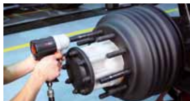
2- Seating drum with sleeves (Composite Impact page 16)
