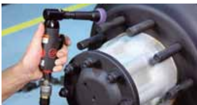
1- Cleaning the drum (Angle grinder page 42)
