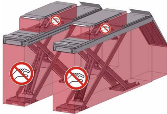
Fig. 3-1 Mechanical danger zones
