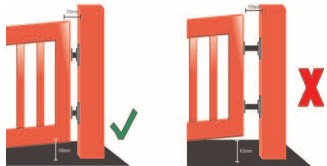
Figure 4 – avoiding gaps over 100mm
