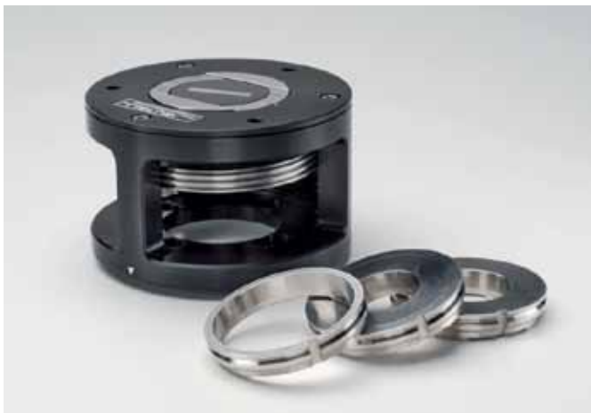
Figure 1b: Grinding specimen holder to hold specimens for cross-grinding rigidly.
