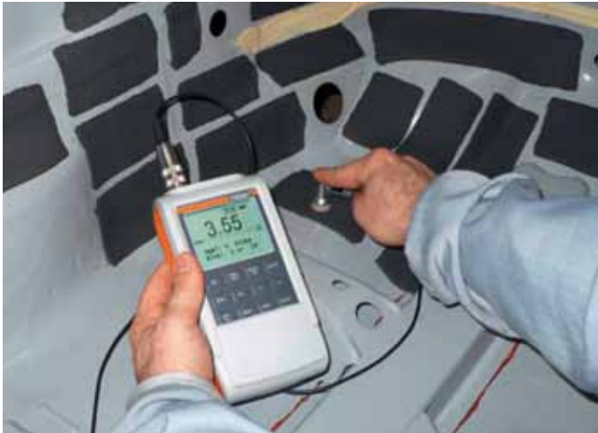
Figure 1: FA14 probe being used to measure SAM coatings (Daimler AG, Mercedes-Benz Bremen factory).
