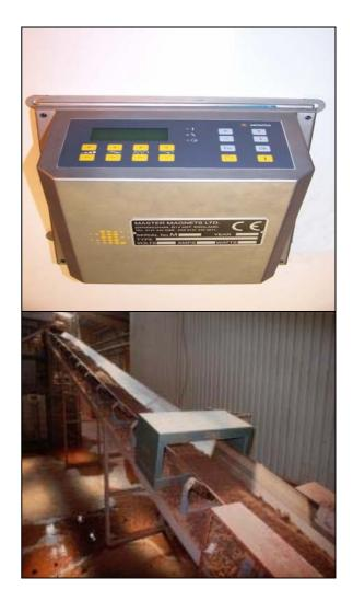
Typical materials examined includes plastics, rubber, glass, clay, fibres, wood, grain, chemicals, coal, cement, food products, powders, liquids and many others for machinery safeguard or protection of the operator or consumer.
