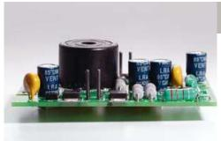
Acoustic device to indicate wrong installation (buzzer).
