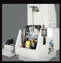
from larger diameter parts. The Model V10 is configured to satisfy the heavy honing requirements of the customer.
