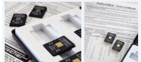
Figure 5. Certified reference materials with thin Au and Pd coatings on Ni/Cu/PCB (with certificate).
