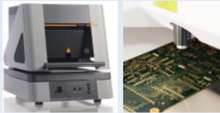
Figure 1. The thickness of Au, Pd, Ni and Cu is measured with a FISCHERSCOPE X-RAY instrument.
