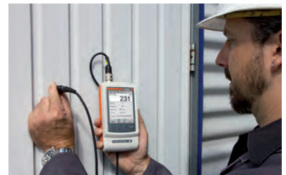
Measurement of paint coating thickness
