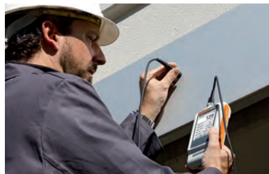
Measurements of anodised aluminum on a façade
