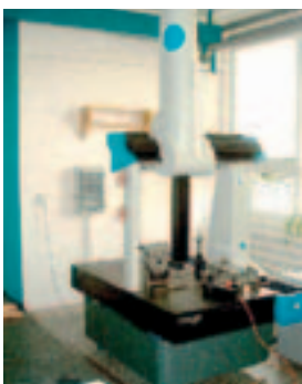
Quality control of dimensions of various parts using DEA GLOBAL IMAGE coordinate table.
