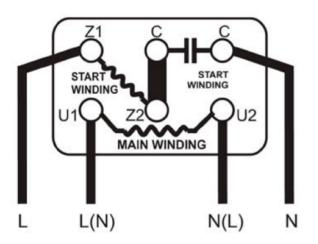
Supply L to Z1 at all times. Supply N to C (top right-hand) at all times.
