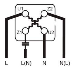
Disconnect the Capacitor cable from U1
