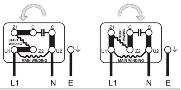
To change direction of rotation simply re-position the 3 metal links in the terminal box.
