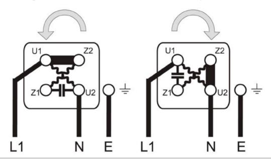
To change direction of rotation simply re-position the metal link and the capacitor.
