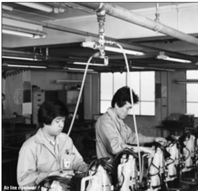
Air line manifold
