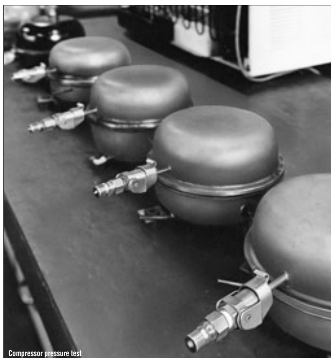
Compressor pressure test
