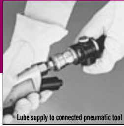
Lube supply to connected pneumatic tool
