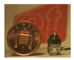
This encoder is just 7.5mm diameter and 10.5mm long yet has A, B, and marker pulse with full TTL square wave. It comes with resolutions up to 360pulses per rev and is affixed to the equipment or instrument by a 6mm nut. The MES-6-P series encoder is ideal where space is at a premium and yet a reliable incremental signal is essential. This new product from Encoder Technology extends and complement their own range of incremental and absolute encoders.
