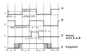
$\begin{array}{lll} \textbf{Incremental signals} & \textbf{TTL square } \underline{\textbf{wave pulses A \& B with}} \\ & \text{compliments } \overline{\textbf{A \& B. B lags A with clockwise}} \\ & \text{rotation (viewed from the shaft end)} \\ \end{array}$
