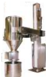
Portable sieve unit supported from Drum Cone valve.
