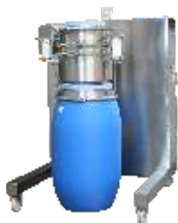
Sieving of APIs into Process Stream.
