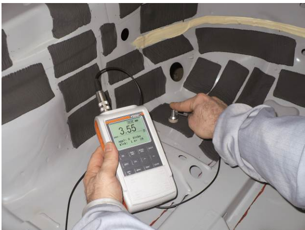
Fig. 1: Locally applied SAM coatings in the passenger footwell, measured with DUALSCOPE® FMP40 and FA14 probe (Daimler AG, Mercedes-Benz Bremen factory)
