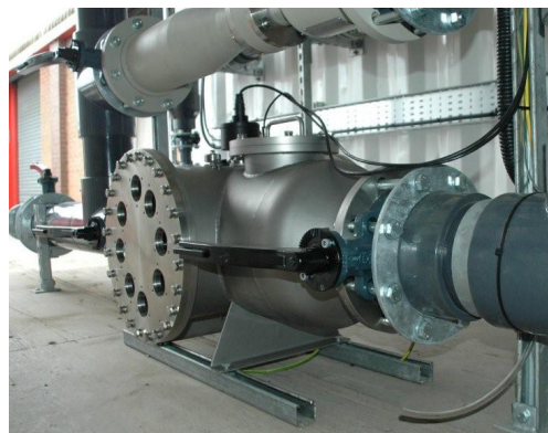
Above: A Medium Pressure atg UV system being validated to demonstrate performance.
