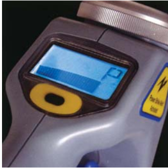
In the P mode the C.A.T 3 detects 'power' signals that are being radiated by loaded cables.
