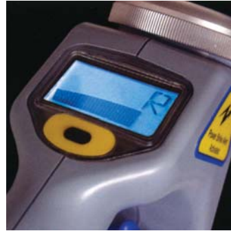
In the R mode the C.A.T 3 detects VLF radio signals re-radiated by buried metallic pipes and cables.
