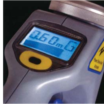
In the G mode the C.A.T 3 detects a tone radiated by the Genny+ to a buried conductor.
