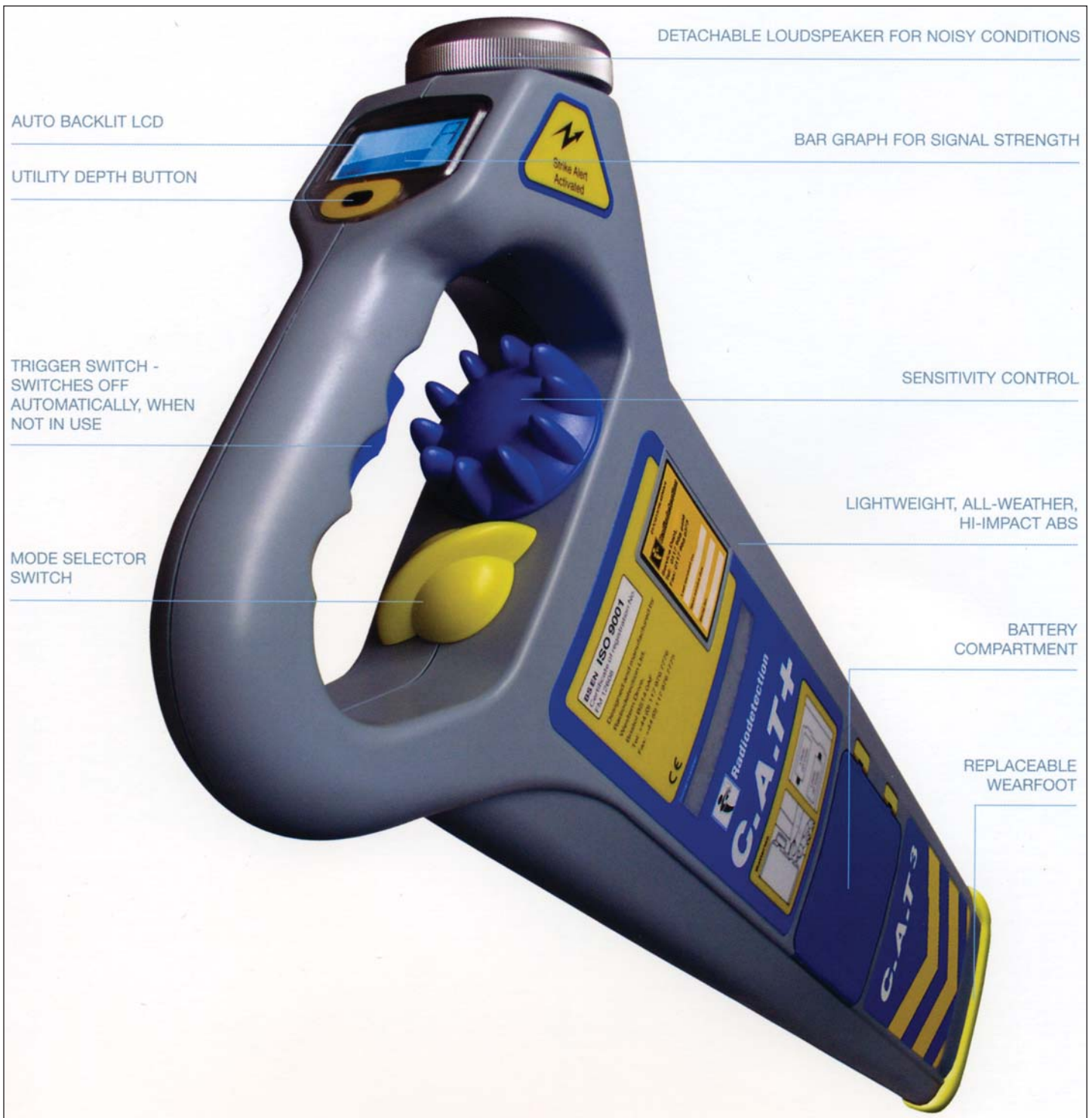
In the P mode the C.A.T 3 detects 'power' signals that are being radiated by loaded cables.
