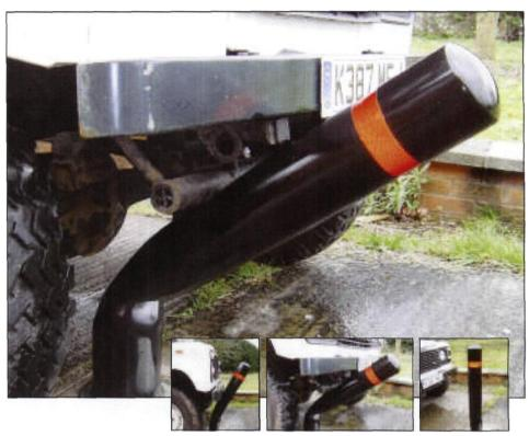
point the bollard will fold through 90 degrees. Once the load is removed the bollard will bounce back to its original upright position. It will continue to fold under a given loading situation an indefinite number of times thanks to the highly durable, resilient polyurethane material called 'Terrathane.
