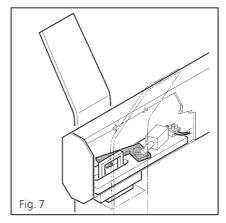
In case of power failure the device locks automatically, as shown in figure 7; the barrier boom can be opened manually as shown in figure 8.
