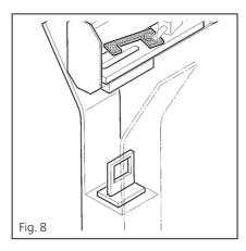
To ensure correct functioning of the lock the barrier boom must not rest heavily on the support pillar. If necessary the locking plate or barrier boom must be re-adjusted.
