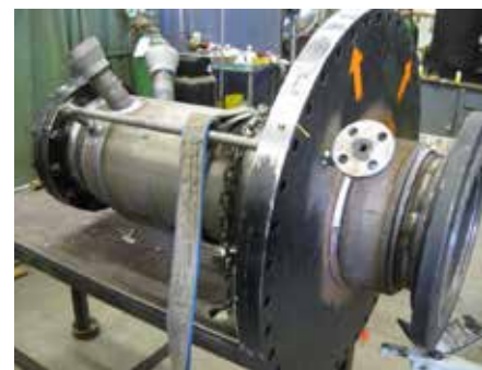
Steam-jacketed fabrication with three spray nozzles installed through the jacket.
