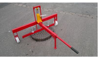
The new light weight hand hydraulic machine has been developed to meet the needs of the vehicle based contractor, who has the need for a low space and low weight machine to add to the "on board" equipment. The machine will fit in the smallest car when dismantled for survey and on site operation.
